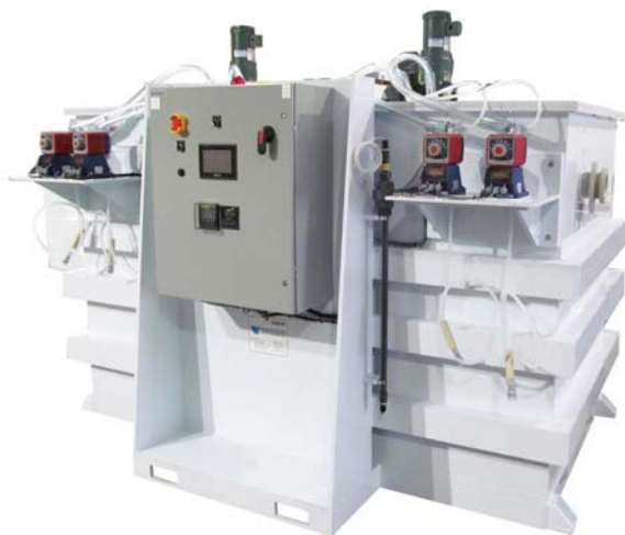
Shown: OMEGA-50-2-SC-G-B-M-IM-1-LR. 50 gpm system, 2 reaction stages, acid and caustic addition, chemical metering pump shelf, 115 VAC IDEC with Maple HMI control panel.
