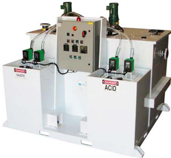
Shown: OMEGA-20-2-DC-G-B-T-IM-1-LR. 20 gpm system, 2 reaction stages, acid and caustic addition, chemical day tanks, 115 VAC IDEC with Maple HMI control panel.
